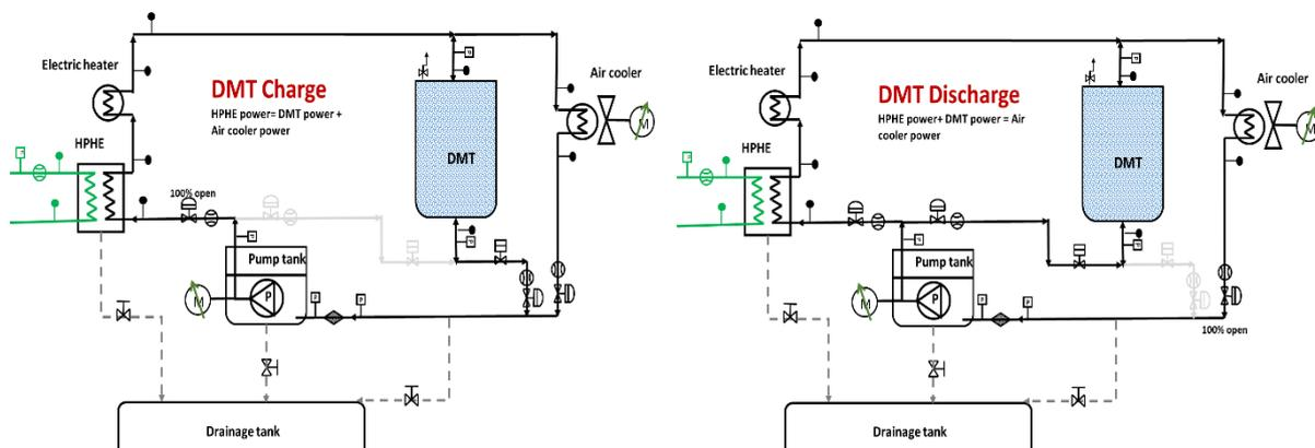
**Figure 2. DMT charge and discharge for a parallel configuration**
