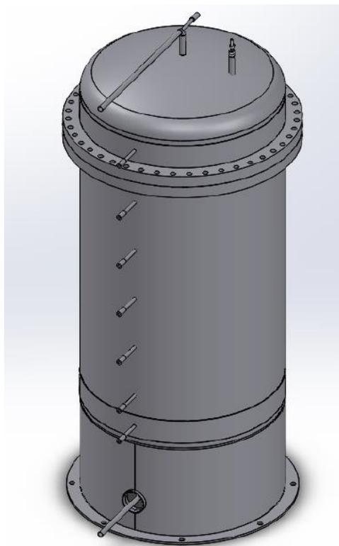
Figure 3. DMT tank and support skirt general view
