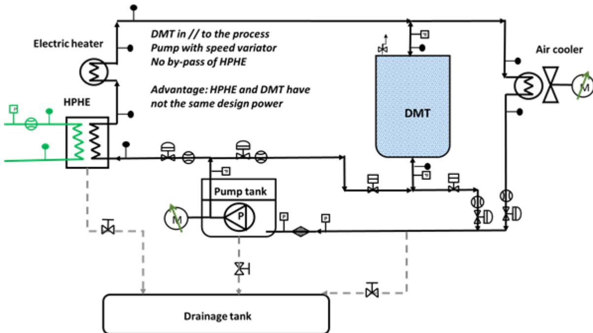
**Figure 1. Scheme of the SMARTREC pilot plant with the DMT in parallel to the process**
